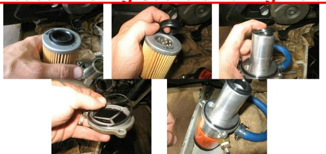
Hose ports are  $\frac{1}{4}$ " NPT and cannot be plugged . If not installing an oil cooler , a line must be looped between the 2 ports . Gauge port is  $\frac{3}{8}$ " NPT . Install adapter with drain hole at the bottom for proper drainage .
